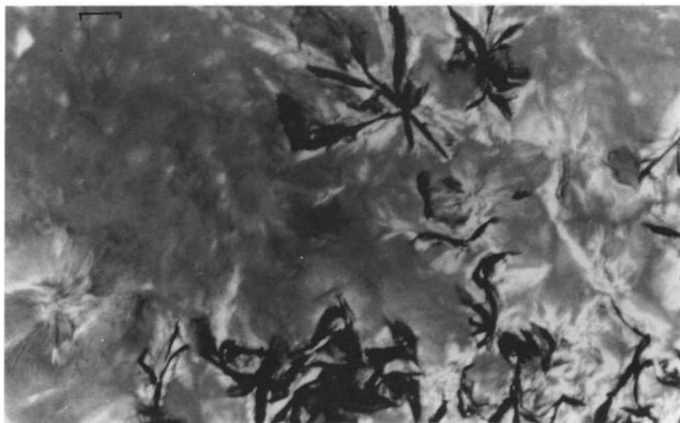
Fig. 3. Photomicrograph of Gelucire 55/18 crystallised from chloroform (scale represents 20 \mu\text{m} , polarized light, red filter).
